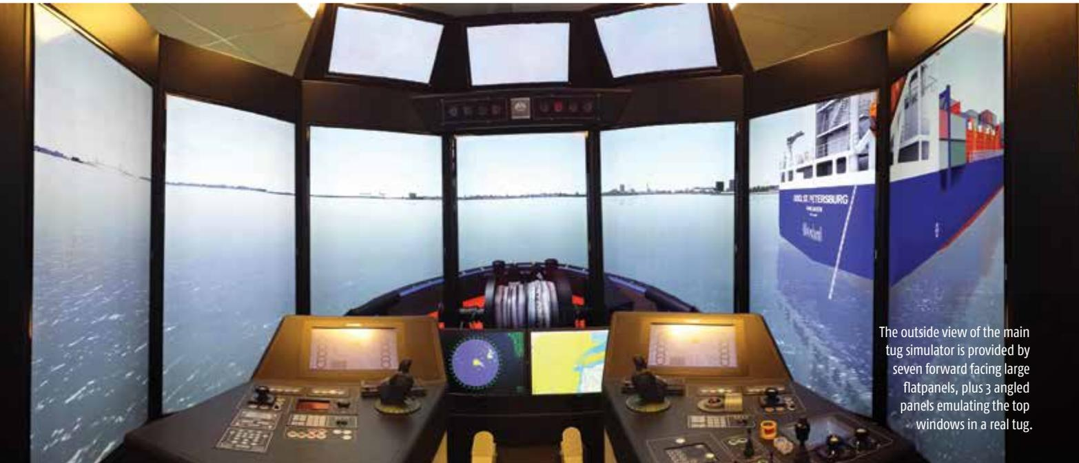
The outside view of the main tug simulator is provided by seven forward facing large flatpanels, plus 3 angled panels emulating the top windows in a real tug.
