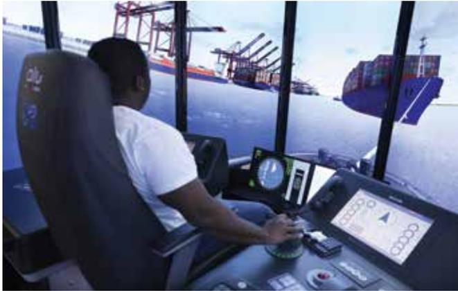
**LEFT:** One of Iskes' tugmasters in the simulator, towing a container vessel in Rotterdam Europort. The main simulator features the same tug bridge console as found onboard the DAMEN 2810 tug for a maximum feeling of realism. **RIGHT:** A desktop tug simulator complements the main simulator at 360-Control. It can be used in the same exercise as the main simulator, or in a separate one.
